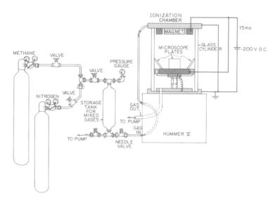
FIG. 1. Experimental apparatus, incorporating Technics "Hummer V" film deposition chamber, used in preparing thin film of Titan tholin on various substrates.
