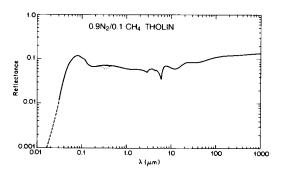
FIG. 5. Normal incidence reflectance calculated using the *n* and *k* values shown in Fig. 4. The dashed line is due to values of *k* extrapolated to shorter wavelengths, as shown by the dashed line in Fig. 4. The dotted curve between 0.2 and 0.4  $\mu$ m is the measured reflectivity plotted in Fig. 3. (See text for details.)
