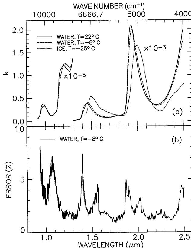
Fig. 2. (a) Imaginary part of the refractive index of water at  $T = 22^\circ\text{C}$  (solid curves), supercooled water at  $T = -8^\circ\text{C}$  (longer-dashed curves), and polycrystalline ice at  $T = -25^\circ\text{C}$  (shorter-dashed curves). (b) Standard deviation of  $k$  for supercooled water at  $T = -8^\circ\text{C}$ .
