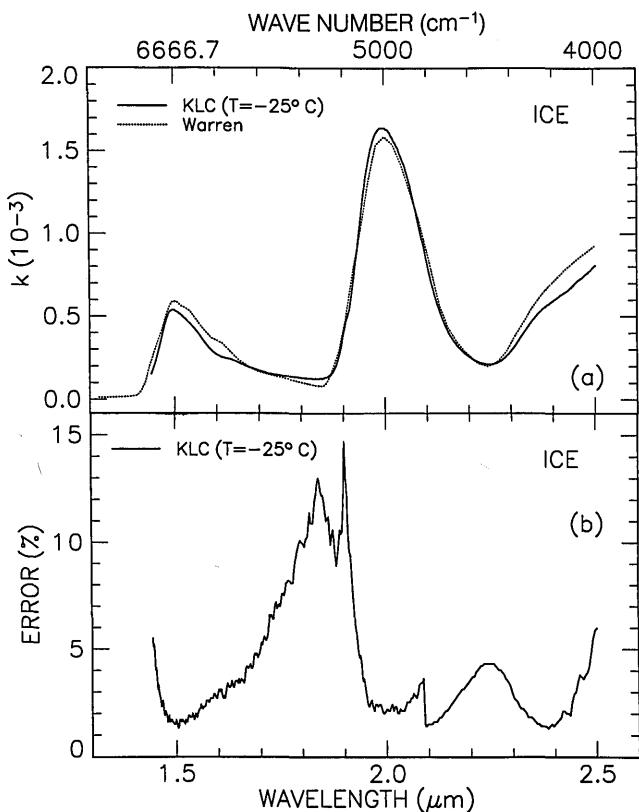
Fig. 3. (a) Imaginary part of the refractive index of polycrystalline ice at  $T = -25^\circ\text{C}$  from the present measurements (KLC, solid curve) and Warren's<sup>10</sup> compilation (dashed curve). (b) Standard deviation on  $k$  for polycrystalline ice at  $T = -25^\circ\text{C}$ .
