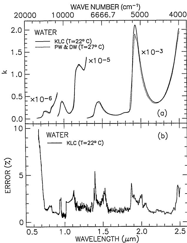
Fig. 1. (a) Imaginary part of the refractive index,  $k$ , of water: the present work (KLC, solid curves) at  $T = 22^\circ\text{C}$  and the PW and DW data (dashed curves) at  $27^\circ\text{C}$ . (b) Standard deviation of  $k$  for water at  $T = 22^\circ\text{C}$ .
