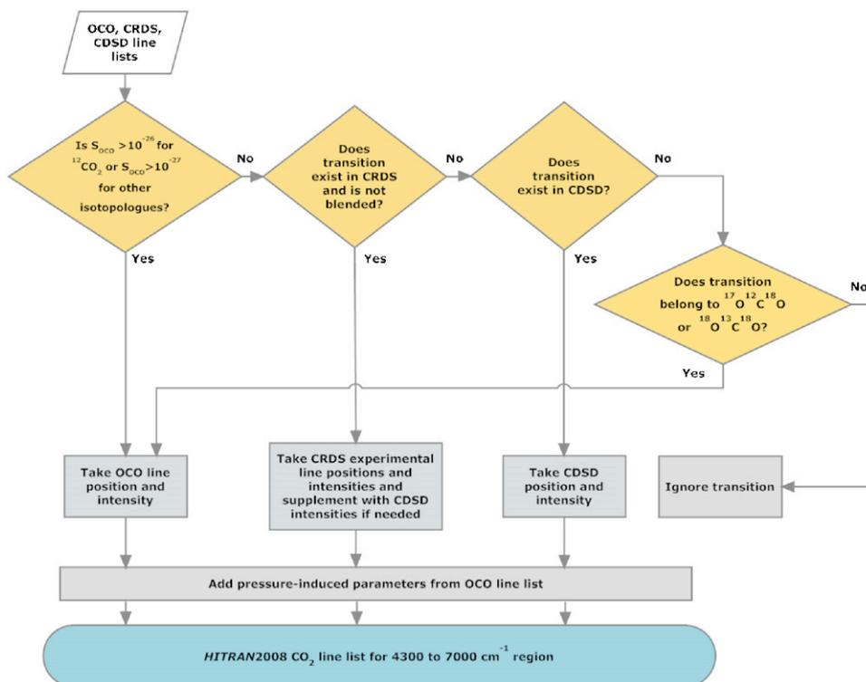
Fig. 1. Flow diagram outlining the assembly of the CO<sub>2</sub> HITRAN2008 line list in the 4300–7000 cm<sup>-1</sup> region.
